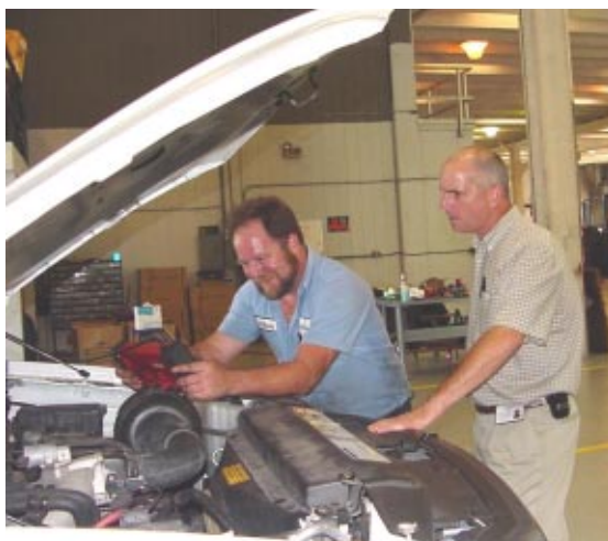
Auto Mechanic Albert Adams (left) uses a hand-held engine analyzer to read problem codes from a sedan that was in for repairs. Superintendent Greg Schmidt observes.
