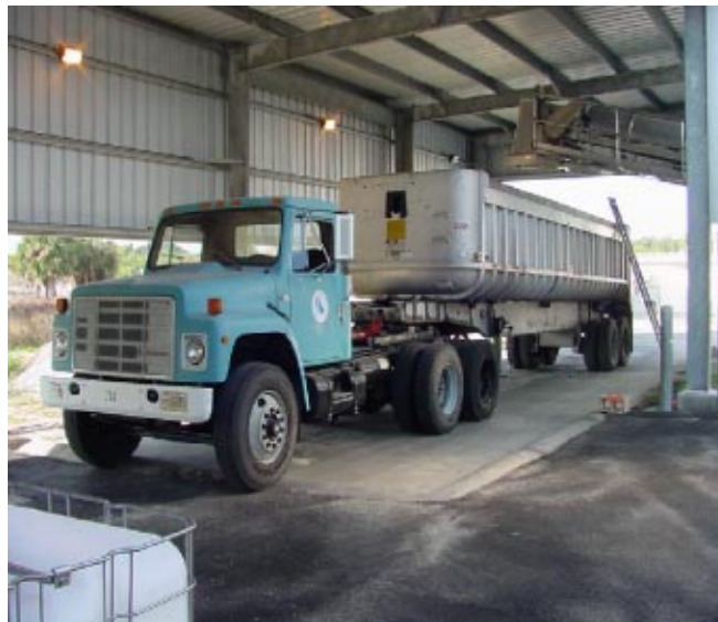
Dried sludge, or biosolids, drop from conveyor belt into truck to be transported to disposal site.
